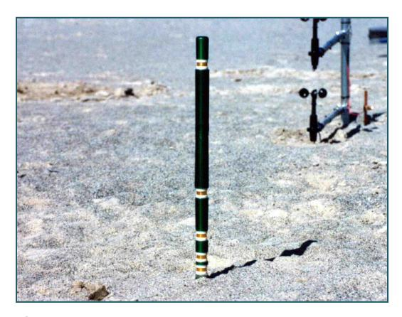
**5 Level Sensit Erosion Sensor 1991**
