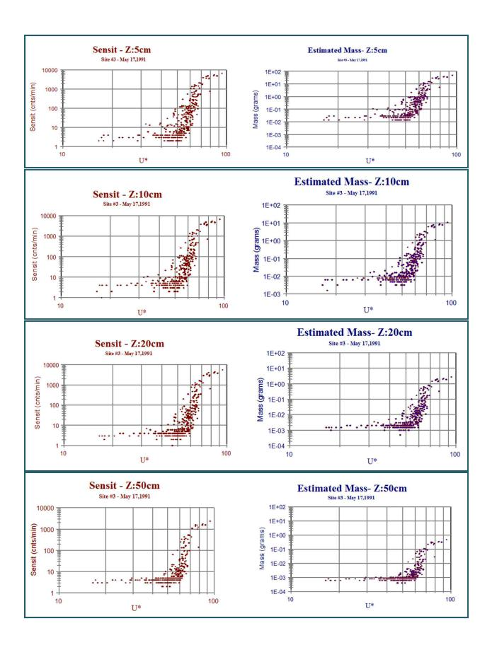
Multi-level data displays a rare look at the vertical profile of simultaneous erosion activity. Log scaling is used to compress highly scattered data. The lowest value data values are Sensit output counts of 1, 2, 3etc. so they appear as a line across the graph. This is just the effect of resolution.
