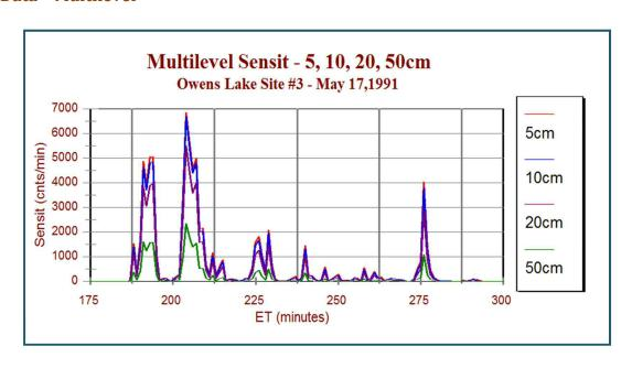
The data graph above was acquired using a 4 level Sensit located at Owens Lake on May 17, 1991. The multi-level sensor is comprised of four separate Sensits housed in a single enclosure where the crystal sensors are mounted vertically on a single post. This simultaneous data was taken at a sampling period of 60 seconds.
